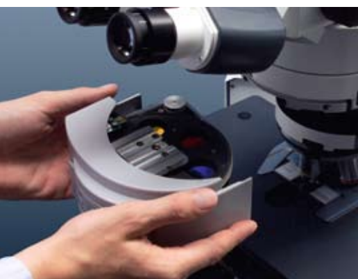
Simply fast: the change from manual to motorized reflector turret
