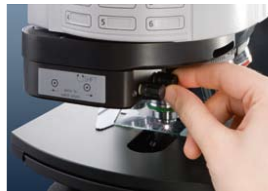
The new motorized DIC turret
