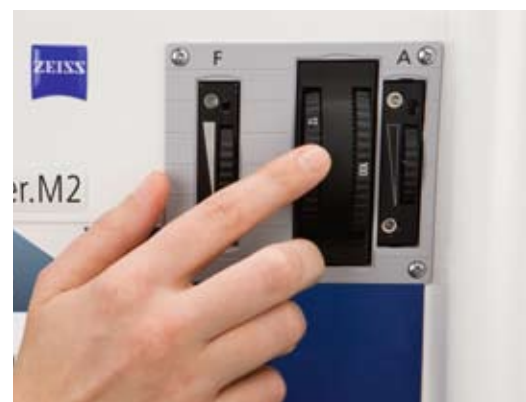
Ideal arrangement of the diaphragm slider and filter wheel in reflected light
